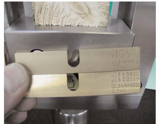
▲ Shims for adjusting clearance of shear line
